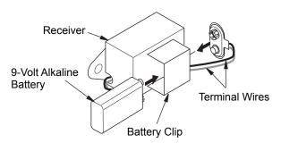
Figure 37 - Attaching Alkaline Battery to Receiver
